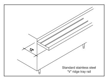
➤ Stainless steel "V" ridge - standard ➤ Flat stainless steel - optional ➤ Plastic laminate - optional ➤ Quartz® - optional
